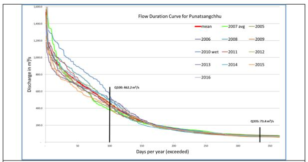
Fig. 5: Flow duration curve and reference flows for the wet and dry season,  $Q_{100}$  and  $Q_{335}$  based on an example from the Punatsangchhu
