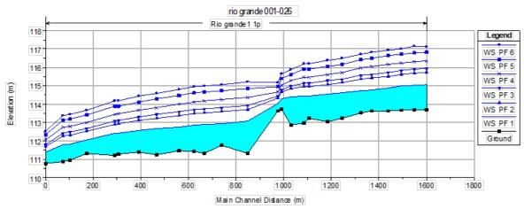
Fig. 11: Calibration of 1D model by means of longitudinal free surface profiles for six different flow rates.
