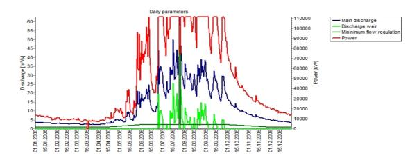
Fig. 32: Results of a CASiMiR simulation of the energy generation for a conceptual HPP on Parochhu
