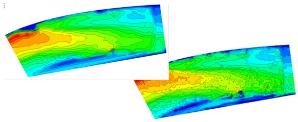
Fig. 9: Comparison of cross section based and scatter point based model of the same river stretch
