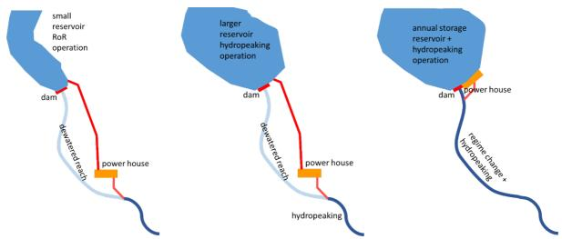
Fig. 2: Types of hydropower plants and river reaches where E-flows are relevant, dewatered reach only (left), dewatered reach and downstream of TRT outlet (middle), downstream of dam (right)
