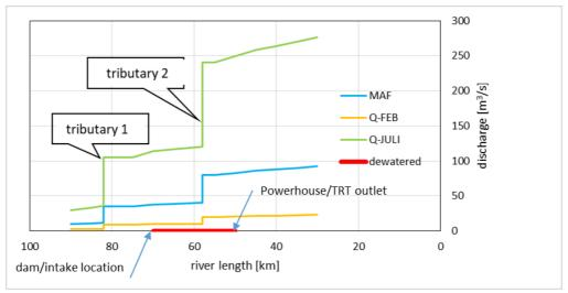
Fig. 6: Example of a simple hydrological longitudinal section of a river with two tributaries.
