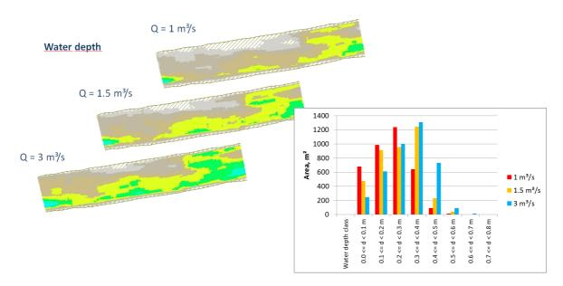
Fig. 13: Visualization and analysis of 1D and 2D model results: example of water depth
