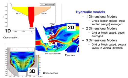
Fig. 8: Flow velocity in different types of hydraulic models
