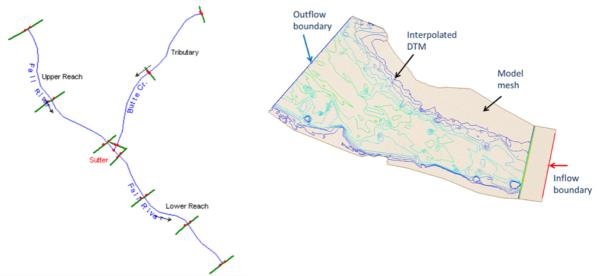
Fig. 10: Setup of geometry and boundary conditions for 1D model (source [HECRAS manual]) (left) and 2D model (right)
