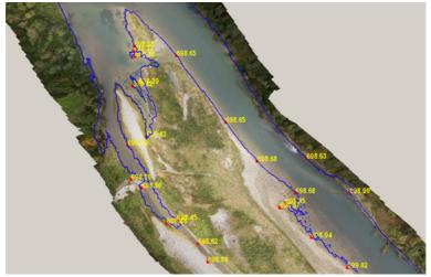
Fig. 12: Calibration of 2D model by means of aerial photo and measured values of water surface elevation
