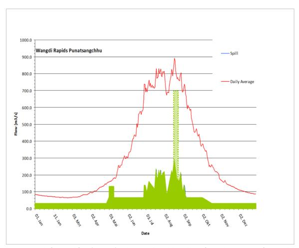
Fig. 35: Example for actual flow (in green) in dewatered reach based on E-flow releases, trigger flows and spill at the dam
